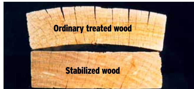
Ecolife's proprietary preservative system improves the weathering performance of Ecolife by reducing cracking, checking and splitting.
